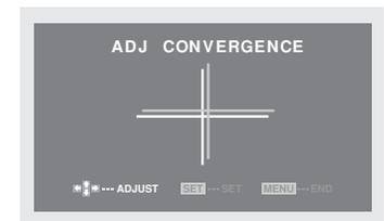
This indicates that the color is misconverged. Proceed to step 4 and perform the adjustment.
