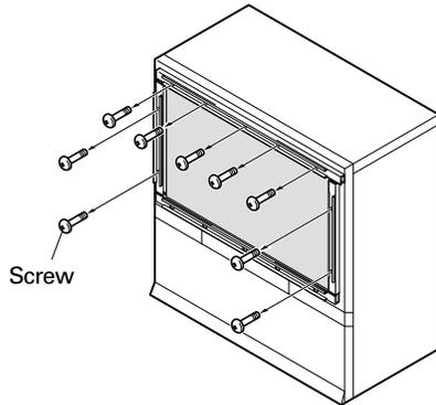
3. While holding the screen in place, remove the upper panel frame and side panel frames.
