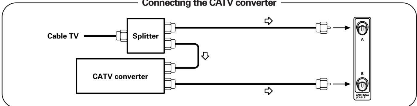
Connecting the CATV converter with VCR
