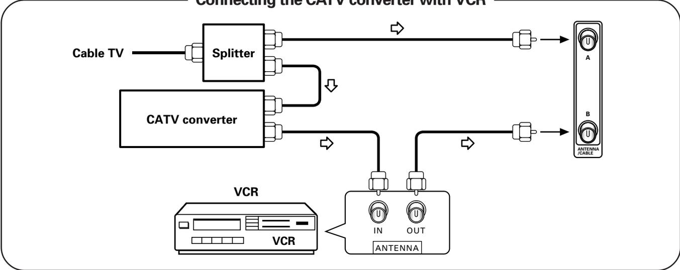
Connecting VHF/UHF antenna and CATV converter
