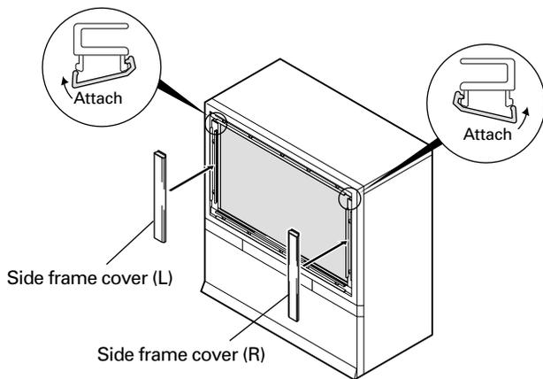
Attach side frame cover along the aluminium edge guards leaving a space of approximately 0 to 1/32 in. (0 to 1 mm) from the upper panel frame.
