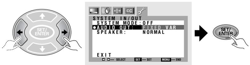
FIXED ..... Signals output from the AUDIO OUTPUT terminal will not change even if the Monitor's volume is adjusted.
