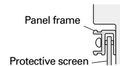
When the protective screen is attached.
