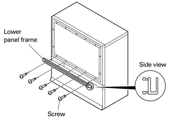
6. Reattach upper, lower and side panel frames as indicated then follow on HOW TO ATTACH THE FRAME COVER.
