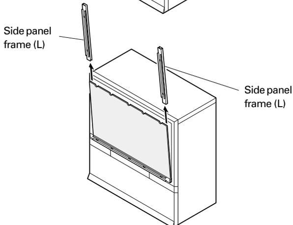
4. Remove the protective screen from the lower panel frame.
