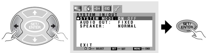
ON ..... The Monitor input is fixed to INPUT 1 and the images of the input source selected by the receiver will be displayed.
